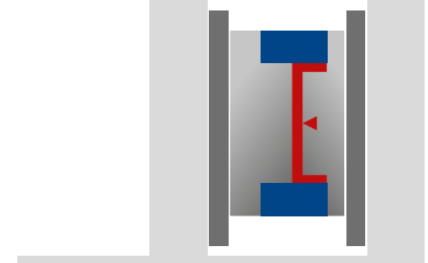
4. Full closing of the tool, and molding by squeezing the melted plastic
